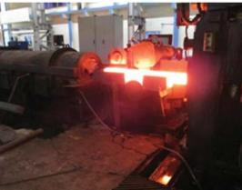
Hot charging of Billets directly from CCM and reheating the Billets through Induction route is becoming a necessity. Billet temperature can be increased by Induction heating and gives the following major advantages:
