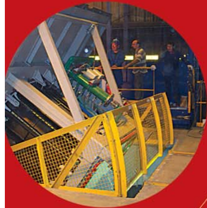
Pit Guard in Operation
