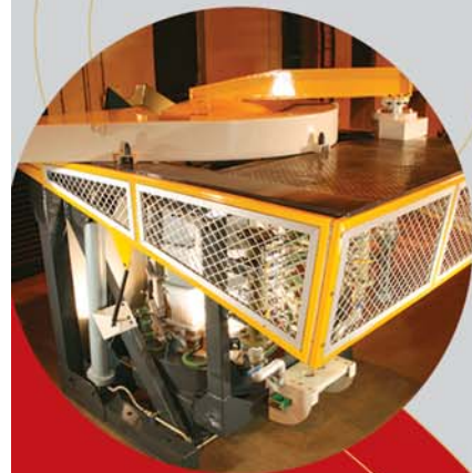
Furnace Lid along with Fume Ring
